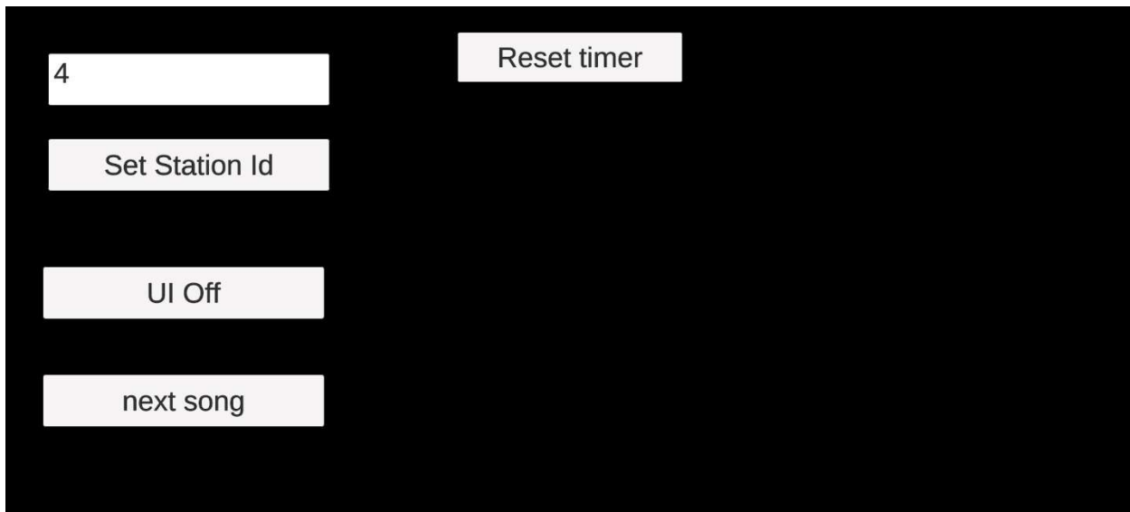
Figure 24. Base station UI. On the top left input field, the user specifies which exhibit this Base station is for. Pressing the "Set Station Id" the base station registers with the database and receives any new interactions that can occur.
